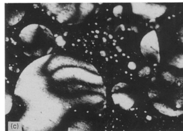
Figure 5 Mesophase microstructures of THE30F pitches after heat treatment in a nitrogen atmosphere at 350 °C for 2 h in the presence of 1 wt % nucleating agents ( \times 160 ): (a) THE30F; (b) THE30F with anthracene; (c) THE30F with acenaphthylene.
